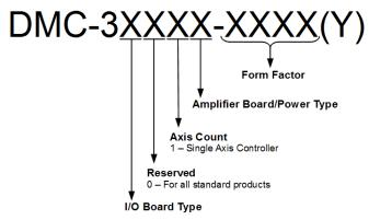
Figure 2: DMC-3x01x Part Number Layout
